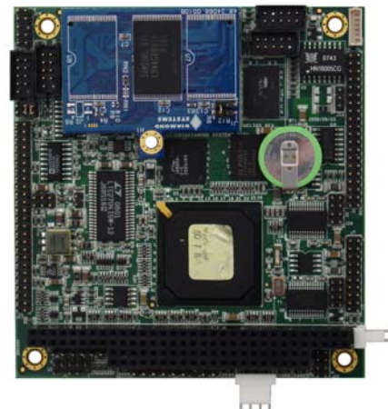
Figure 6. FlashDisk Installed on Helios
